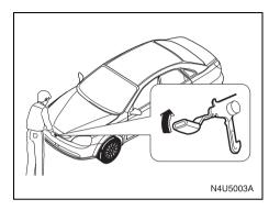
2) Then go to the front of the vehicle and lift the bottom of the secondary hood release lever upward. The secondary hood release lever is located near the front center of the hood.
